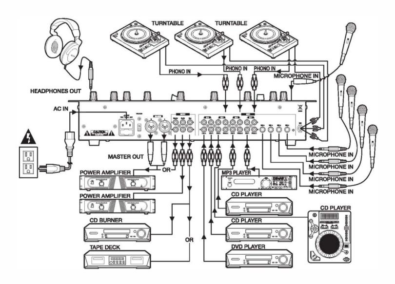
This mixer permits connection of up to thirteen (13) audio input sources, including five microphones. Such a system might include, for examples:
